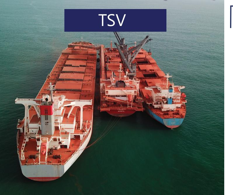
TSV are designed to transfer cargo from a vessel to another one.
