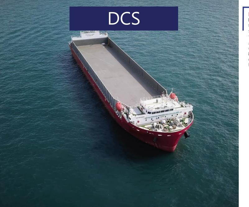
DCS are able to sail **much faster than traditional sets of barge and tugs** while generating substantial savings on fuel thanks to economies of scale and optimized bodylines. They are self-propelled by either fuel or LNG main engines.
